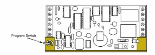
From inside the enclosure, turn the setup toggle switch to ON and then press [7] on the keypad
