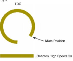
as shown, N/O contacts held closed. Actually, the high speed relay is turned 'OFF' 1/2 inch plus the DRIFT factor before the ram reaches the "MUTE" position.
