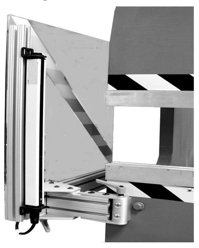
NOTE: The machine mounts can also be secured to the outside of the machine bed. However the method shown aligns the the light beams more acurately.
