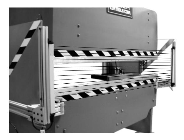
The swing out feature is for loading and unloading dies from the end of the press. Simply loosen the allen locking screw and rotate the brackets to the front of the machine. This clears the end of the press for accessibility.
