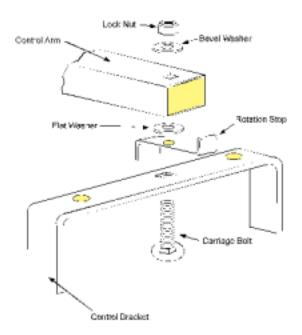
You Can Also Mount The System IIe On Top of the Bracket
