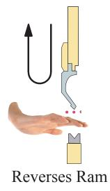
The laser beams (see BOX BENDING mode) are active when the ram is descending, should the beam be broken before it reaches within .100 of the part being formed the machine will be immediately reversed.
