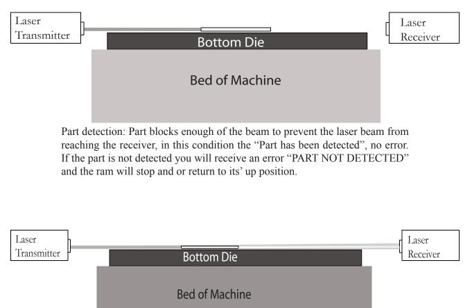
If you are forming small thin parts, always teach the Laser Sentry the part surface with the part in the same place where you are going to form the part.
