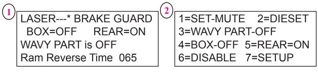
This is the screen seen when in normal running mode. Press the MENU key. This screen will appear. Press [1] for QUICK MENU.
