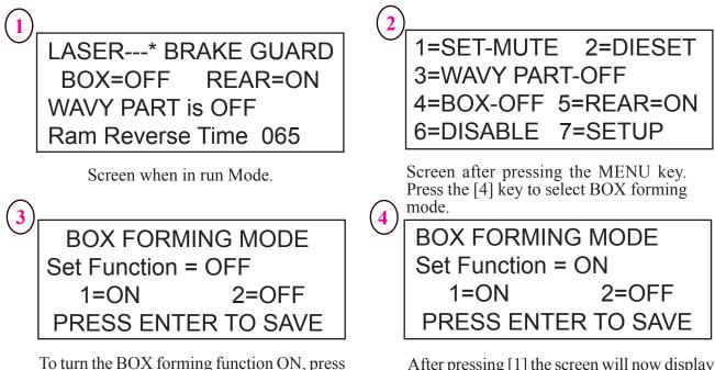
After pressing [1] the screen will now display "Set Funtion = ON". Press the [ENTER] key to save the function. Press [SKIP] to return to the run mode.
