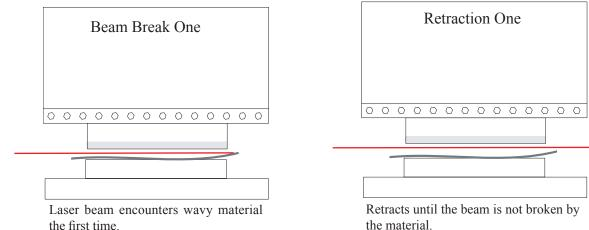
For the ram to retract only until the laser beams are no longer broken you must set the RAM REVERSE function in the SET UP menu to PART(ial) return.
