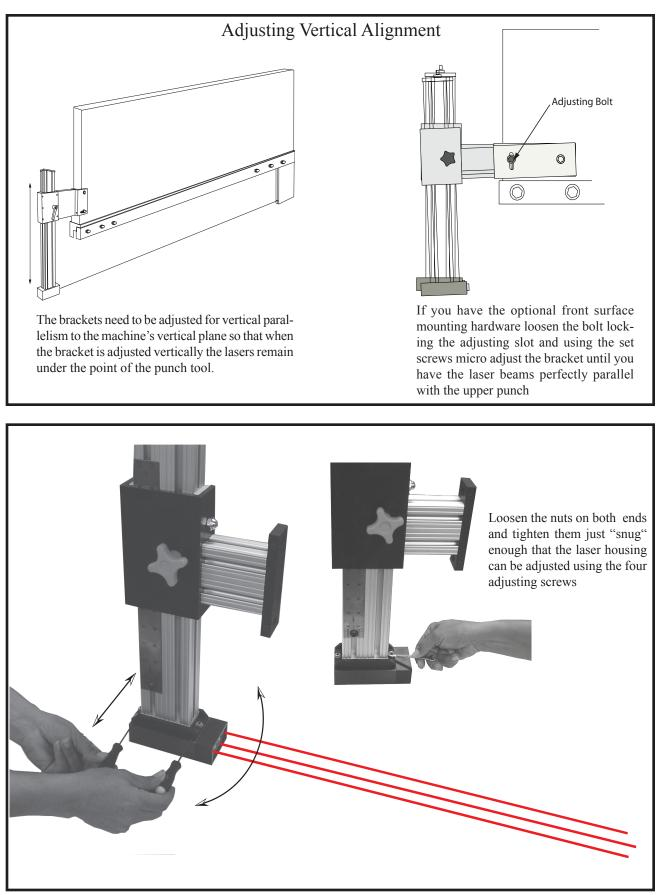
By loosening the nuts slightly you can micro-adjust the skew of the beams. Using two allen wrenches loosen the micro adjusting screws in the direction you want to move the head and tighten the opposite screws until reaching correct alignment. Tighten the opposing screw and recheck alignment. Micro-adjust the screws until you have perfect alignment and both screws are "snug" tight.
