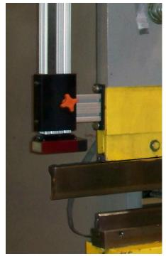
Mount the brackets so that when it is raised, the die can be safely removed without interference with the laser bracket and laser housing.
