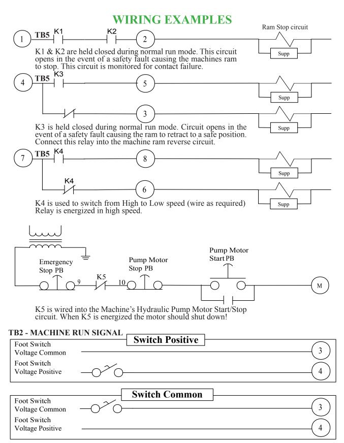
**Machine run signal** - Input from a foot switch circuit or ram closure valve circuit. (TB2) Terminal #3 & 4: The Board is supplied with a AC input module installed (Yellow). This module uses 90 to 140VAC/VDC. Connect the Common to TB2 (3). Connect the Positive from the N/O circuit to TB2 (4). If you require a DC input, install the (White) DC module. Wiring is the same except it requires 3 to 32VDC.
