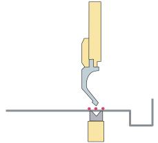
When the ram is descending, the machine is guarded by the *Laser Sentry*. At 1/2 inch or greater above the part being formed, the *Laser Sentry* shifts the machine's ram into slow speed. (down acting machines).
